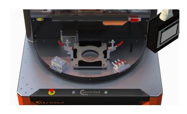
Equipment Dimensions: H: 2100mm W: 1360mm D: 1360mm Weight: 700Kg - Approx.
